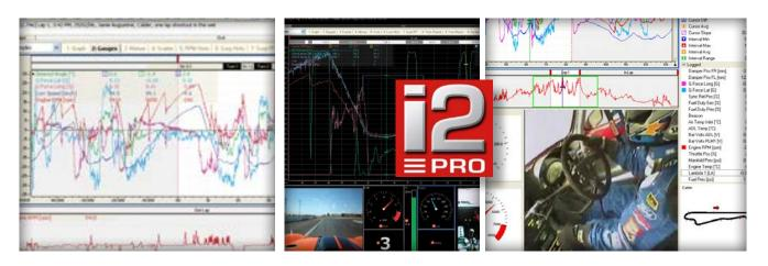
MoTeC's i2 Pro Data Analysis software includes new Feature Licences that can be purchased to activate a particular feature on one physical computer for a nominated length of time. The first features released include Licences to analyse non-i2 Pro log files using i2 Pro and a Licence to manipulate log files via an API (Application Programming Interface).
